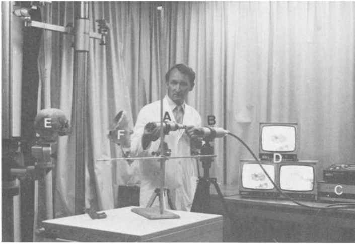
FIG. 18— Setup of the video comparison apparatus: two video tubes (A and B), electronic and mixing units (C), three monitors (D), skull in question (E), and impression of the face of Pestalozzi in clay (F).
